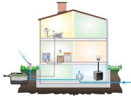
CT-SS: Composting toilet with septic system
