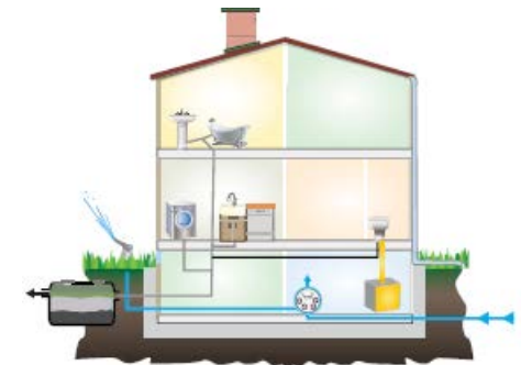
UD-SS: Urine-D toilet with septic system
