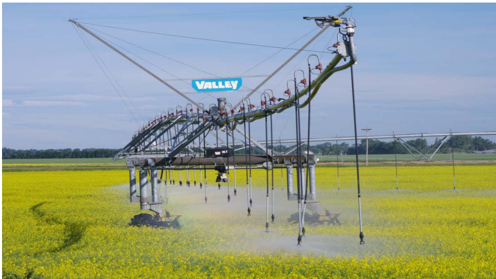
Figure 3. Low pressure pivot showing much reduced exposure of droplets to evaporative forces.
